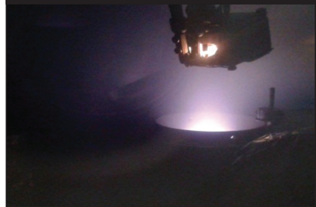
Figure.: In this figure, during sputter process, target-substrate position can be observed.
