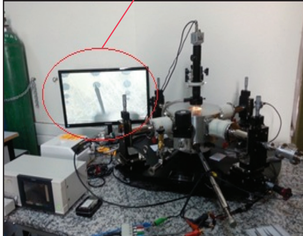
Figure. : probe station and impedance analyzer near by. On the screen, sample contact points can be observed from the top view of the sample.
